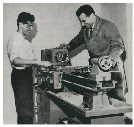
room that can be found in industry. With a heavy duty engine lathe, milling machines, bending machines, drill presses, rolling machine, shears and a grinder, almost any conceivable job of shaping and cutting metal can be performed.
